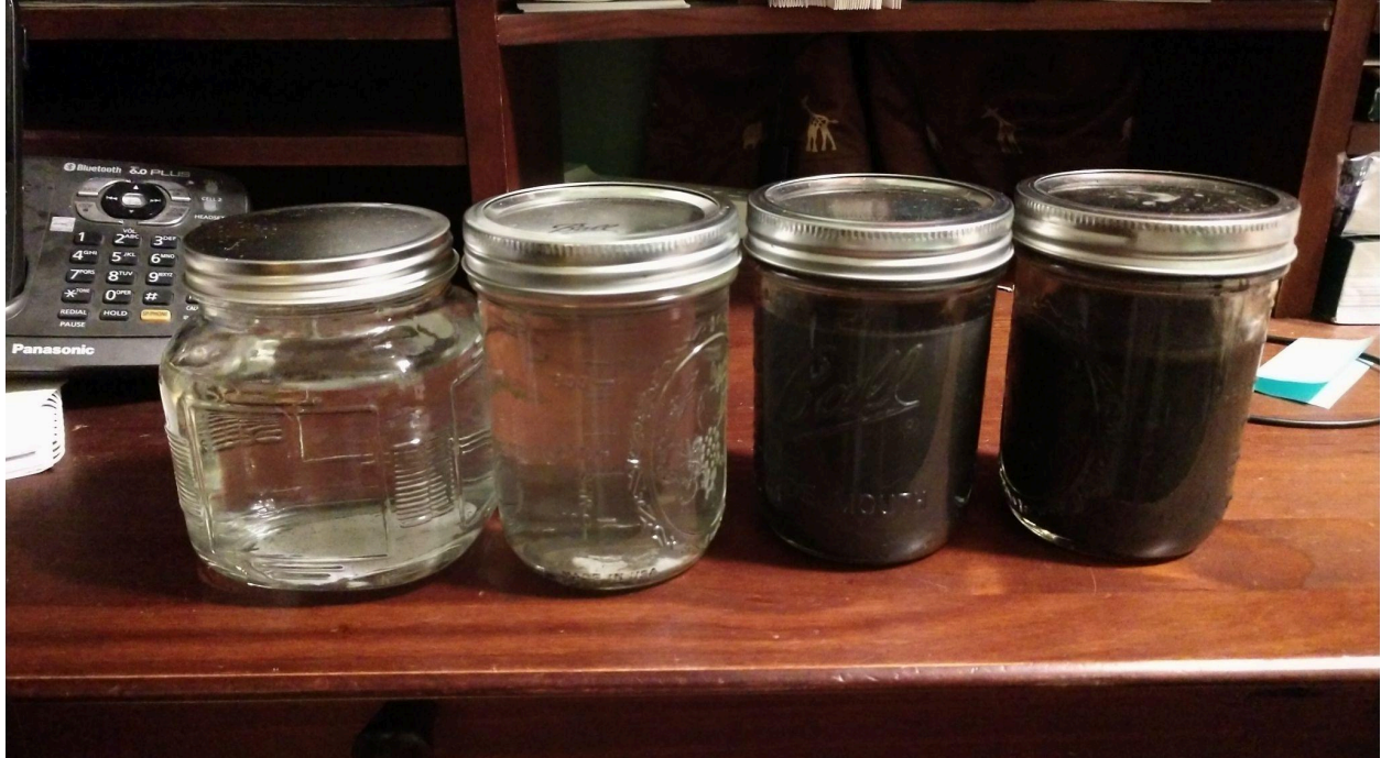
Figure 3. Water samples taken from Mahanoy Creek in February 2018 both upstream (left) and downstream (right) of coal refuse reclamation activity. Sediments in water are mostly coal fines.
